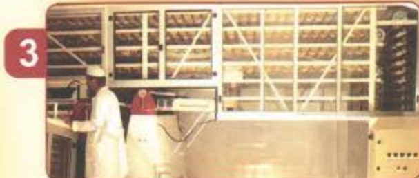
Basket's conveyor for first proofing.
