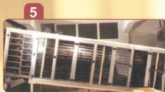
Belts conveyor for second proofing of the shaped disks
