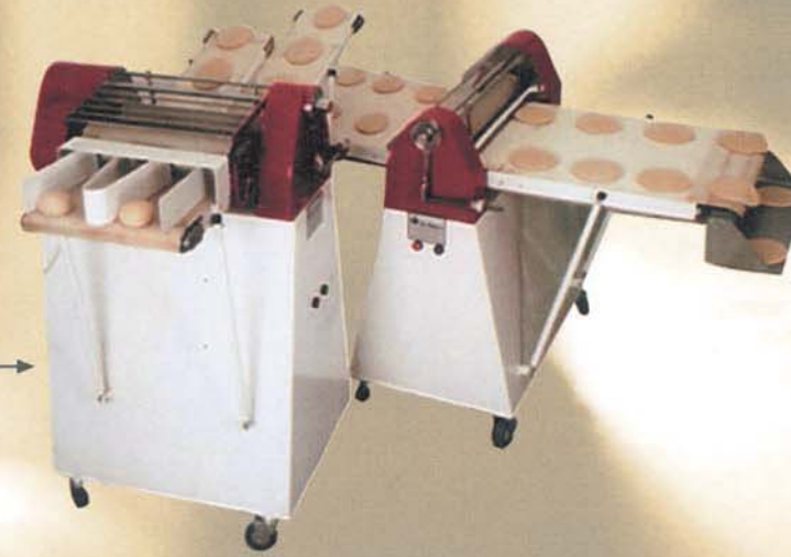
Flattening machines with adjustable rollers for the flat bread sizes control
